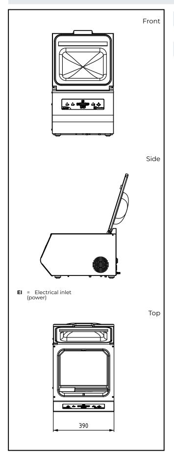
Electric Supply voltage: 220 V/1N ph/50/60 Hz **Total Watts:** 0.7 kW Key Information: External dimensions, Width: 390 mm External dimensions, Depth: 502 mm External dimensions, 345 mm Height: Net weight (kg): 33 Pump:  $8 \text{ m}^3/\text{h}$ **Useful chamber size:** 326 x 240 x 118(H) mm
